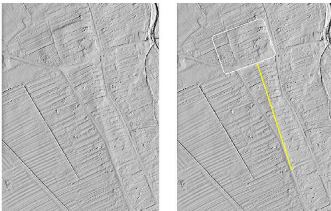
Fig. 4. LiDAR survey (left) and interpretation (right) of the fort and civilian settlement, revealing the outline of the fort (white) and a road segment (yellow) (12/2018) [©MNIT].
